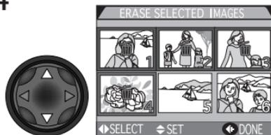
Press multi selector up or down to select image for deletion. Selected images are marked by icon. Repeat steps 3 and 4 to select additional images for deletion. To deselect image, highlight and press multi selector up or down. To exit without deleting images, press MENU button.
