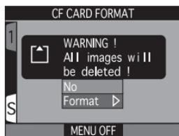
Highlight **Format** (to exit without formatting card, press MENU button or highlight **No** and press multi selector to right)
